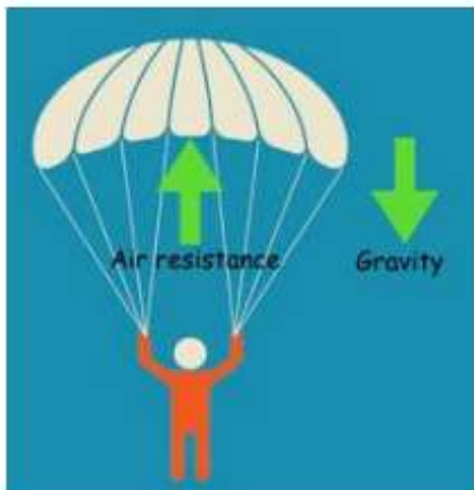
Air resistance slows down the parachute as gravity pulls it to the ground.
